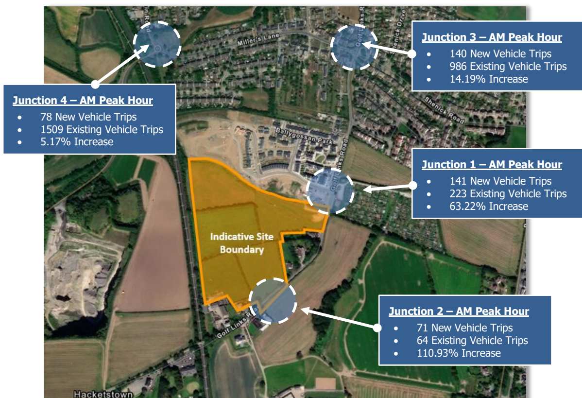
Figure 7.1: Increase in Vehicle Trips Generated Through Key Off-Site Junctions (DS 2039 AM Peak)
